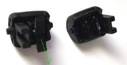
by itself). When assembled, the white counterpart in the other half of the housing pressing on it with a spring. Simply pull out the bracket (see photo) of the old button wheel and put it in the new one.
