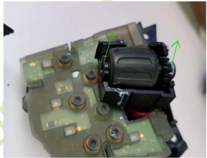
Then you can start assembling. Put the button wheel back in its holder and check for correct function. Put the housing back together and screw together.
