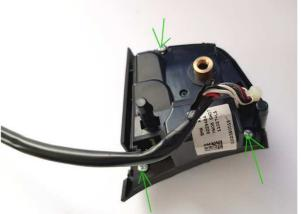
Carefully separate the two housing halves from one another.
