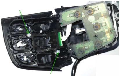
Now release the button wheel itself from its holder. To do this carefully and pry out the nose on one side and then on the other so that you do not damage the bracket.
