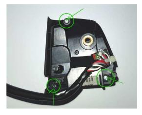
The button wheel with its holder is screwed inside again. Unscrew these two screws as well.
