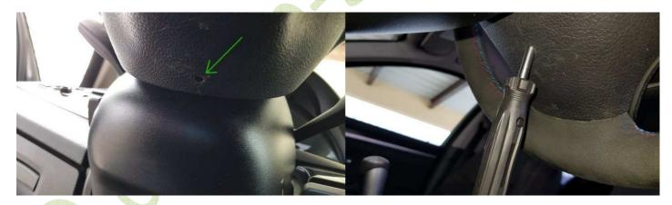
There is a small round opening under the steering wheel, into which e.g. with a small flat screwdriver. The airbag lock is located under the opening. By pushing up, the clasp with which the airbag is locked releases and you can fold
