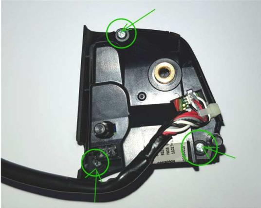
As with the right switch unit, there are 3 screws on the back, unscrew them to open the switch unit.
