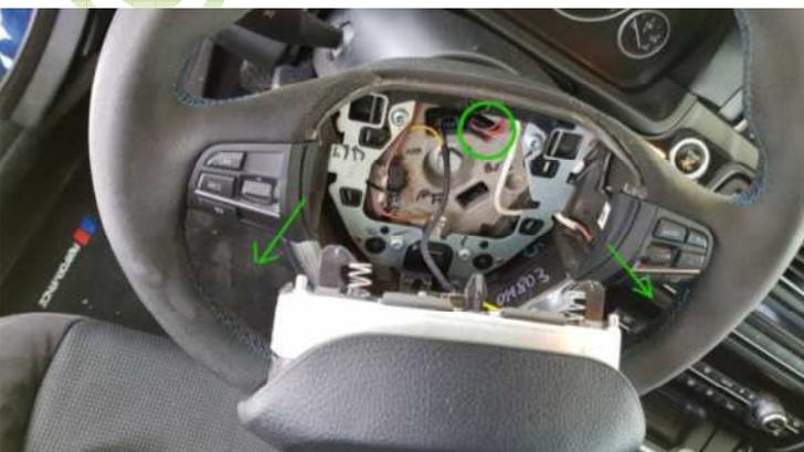
*Note: Depending on the year of construction and model, the locking mechanism can be slightly different. For example, many steering wheel models have 2 locks on the side at the bottom. The principle is always the same.*
