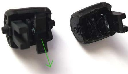
Carefully push the new button wheel back into the holder and tighten it in the housing with the two screws. Now screw the housing together again with the 3 screws on the outside.
