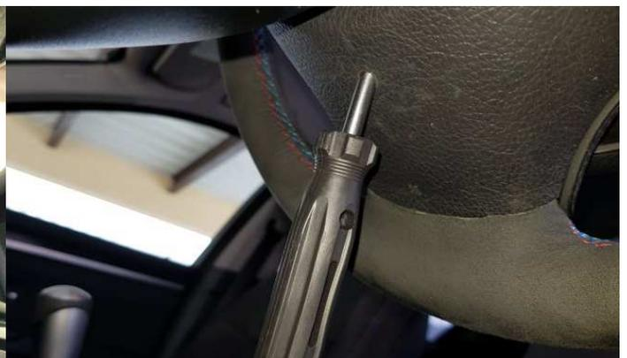
There is a small round opening under the steering wheel, into which e.g. with a small flat screwdriver. The airbag lock is located under the opening. By pushing up, the clasp with which the airbag is locked releases and you can fold it out to the front. Hold the screwdriver as vertically as possible so that the lock is caught.
