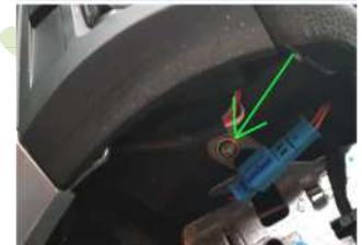
At many models (F25 etc.) the clasp from the steering wheel is screwed to the button units. In this case you should remove the key units together with the clamp. This is usually not only screwed to the switch units, but also screwed in the center of the back of the steering wheel. In this case, first unscrew the screws from the rear so that the cover can be taken down together with the switch units.
