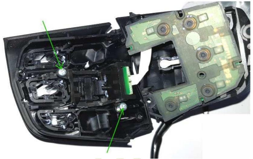
The button wheel with its holder is screwed inside again. Unscrew these two screws as well.
